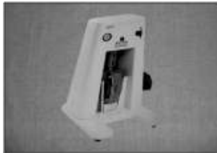
Fig.5 : Cartridge Containing Molten Lucitone Frs Placed On To The Success Injection Unit
