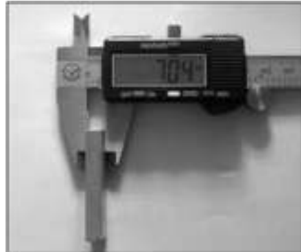
Figure-6: Measurement Of thickness Of The Specimen
