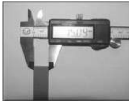
Figure-5: Measurement Of width Of The Specimen
