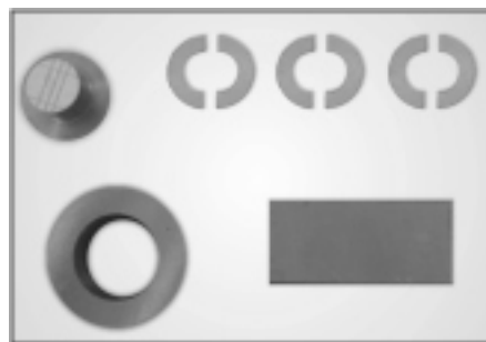
Fig.VI: Split mold assembly A. Master die with reference lines B. Split molds of different heights C. Outer circular ring D. Flat rectangular metal plate
