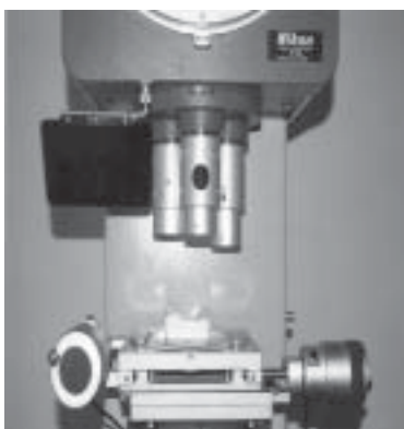
Fig 3 Nikon profile projector microscope
