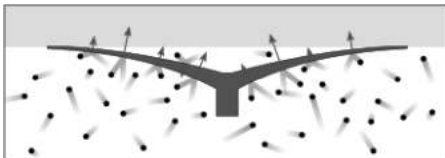
Fig 1 : Pressure On A Suction Cup As Exerted By Collisions Of Gas Molecules That Holds The Suction Cup In Contact With The Surface.
