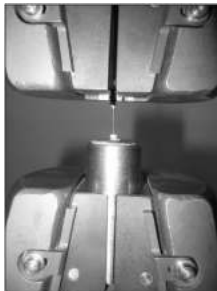
Fig. 1: Loading Of Specimen To Fracture
