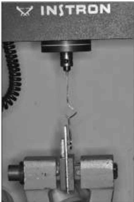
Figure 4: Specimens positioned in INSTRON for shear testing.
