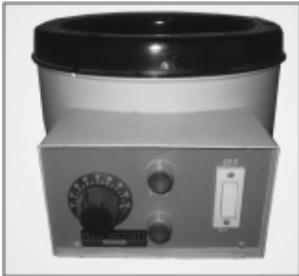
Fig. II: Hot water bath
