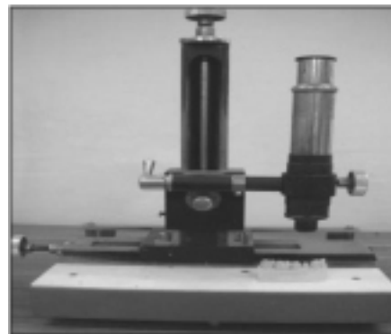
Fig. 7 - Sample Testing Under Travelling Microscope
