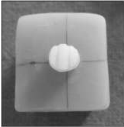
Fig. 4 Ridge lap surface modified by vertical grooves
