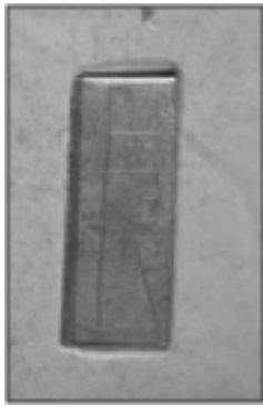
Fig.1. Putty impressions made with brass mould
