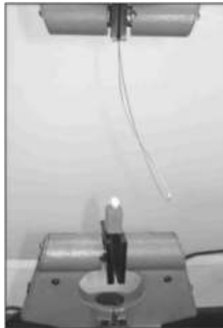
Fig 5: Debonded Bracket From The Labial Surface Of The Tooth
