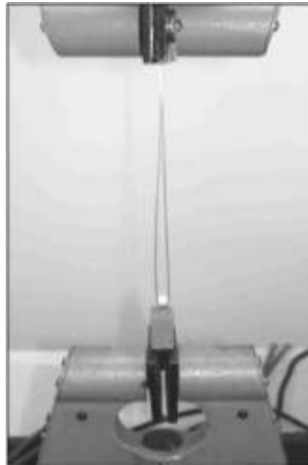
Fig 4: Force Application Parallel To The Labial Surface Of The Tooth
