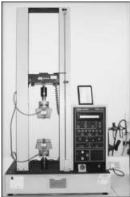
Fig 3: Instron Universal Testing Machine
