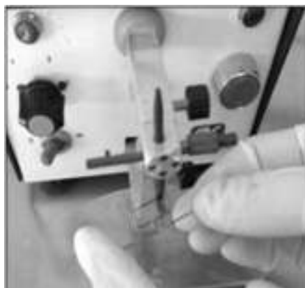
Figure 4 : Spot Weld The Stainless Steel Mesh To The Grid Framework
