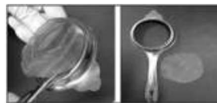
Figure 1 : Mesh Being Cut Off From Commonly Available Stainless Steel Tea Strainer
