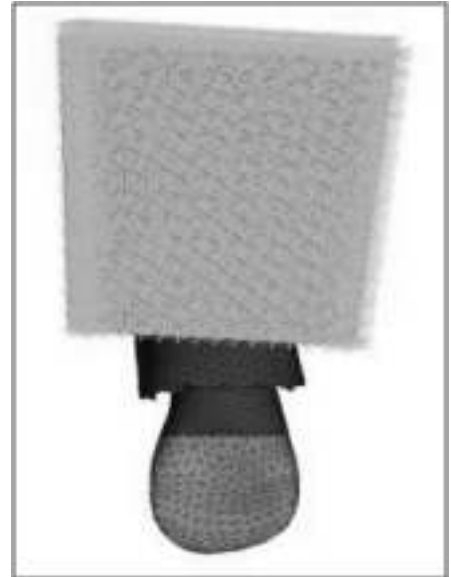
Figure 4 3d Model Of Maxillary Central Incisor With Post And Core Assembly And Applied Boundary Conditions.
