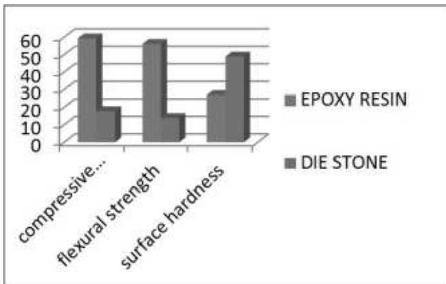
Bar Chart -2: The Compressive Strength, Flexure Strength And Surface Hardness Of Epoxy Resin And Die Stone
