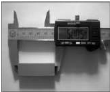
Figure-4: Measurement Of length Of The Specimen
