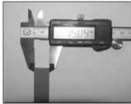
Figure-5: Measurement Of width Of The Specimen
