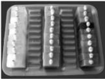
Figure 1 – Sample After Brackets Bonding, Group-1: Bracket Bonded With Transbond Xt (3M- Unitek, Monorvia) .
