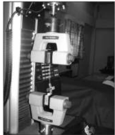
Figure 3 – Instron Machine With Mounted Testing Samples For Shear Bond Strength Testing
