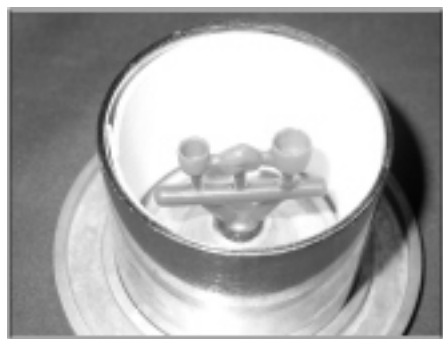
Fig 2. Completed Wax Pattern To Be Invested In Metal Ring With Ring Liner
