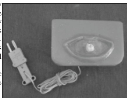
Figure 4: Prepared molar with thermocouple
