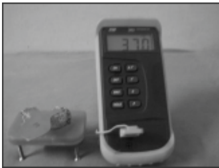
Figure 6: Prepared molar with thermocouple with digital thermometer
