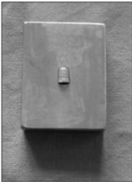
Figure .6 : Custom made stainless steel coping holder with coping
