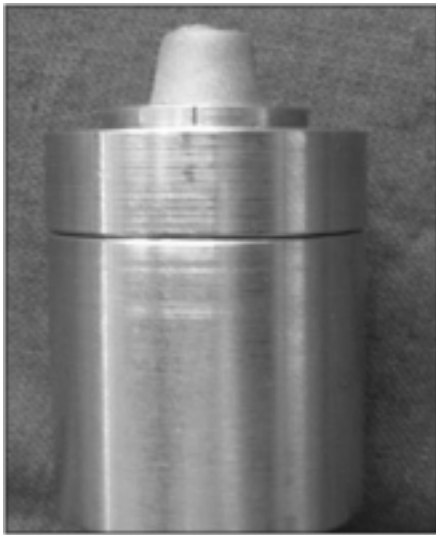
Figure .5 : Cast coping seated on the master die
