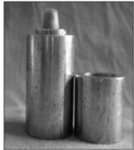
Figure. 4 : Resin pattern on the master die
